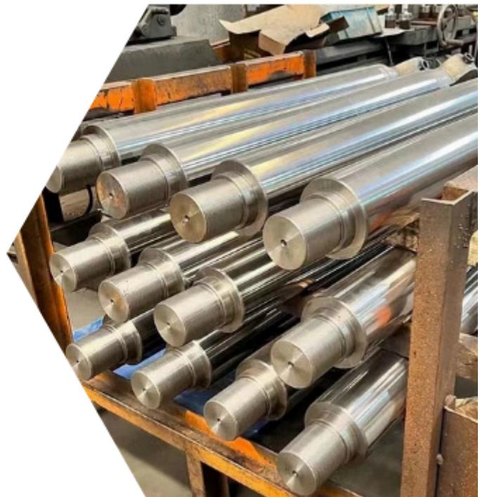
**Hard Chrome Plated Rods** are steel rods coated with a robust layer of chromium that significantly enhances surface hardness, corrosion protection, and smooth operation. These rods are ideal for heavy-duty applications in hydraulic systems, industrial machinery, automation equipment, and more. With tight dimensional tolerances and a polished surface finish, Baokun's chrome rods ensure optimal performance and compatibility within precision assemblies.
